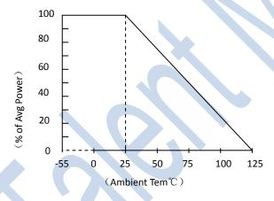
The power of termination will change with ambient temperatures. At higher temperatures the power will descending linearly.
