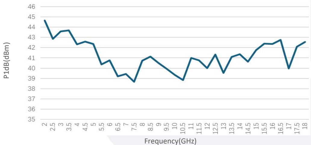
P1dB vs Frequency
