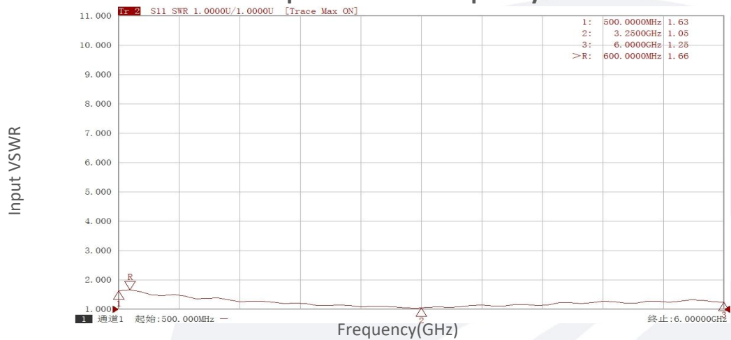
Input VSWR vs Frequency
