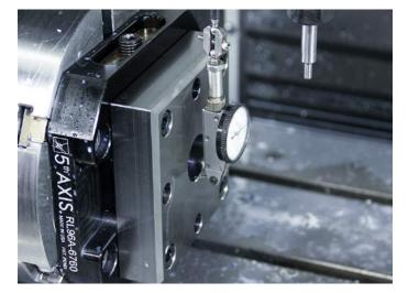
Precision center bore allows for indication of rotation.
