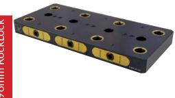
Size: 158mm x 338mm x 30mm Spacing: 2x M12 or 1/2" SHCS @ 96mm or 250mm Material Construction: Aluminum (RL96A-3613S1)
