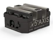
Size: 125.7mm x 152.4mm x 72.9mm Jaw Set Material: Hardened Steel 3 Piece Master Jaw Set with Serrated / 45° Dovetail Jaw Width: 75mm Max Torque: 75 Nm Forward Clamping Range: 0 - 28.5mm Reverse Clamping Range: 31mm - 64.2mm Fixed Jaw Forward Clamping Range: 0 - 75.9mm Fixed Jaw Reverse Clamping Range: 56.8 - 147.3mm
