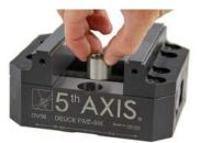
**Removing Center Jaw** The center jaw is bolted through the base and held in position with precision bushings.
