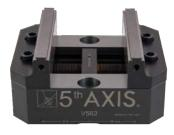
Size: 5" x 6.0" x 2.9" Material Construction: Jaw Width: 4.95" Forward Jaws Clamping Range: 0 - 3.61" Reverse Jaws Clamping Range: 2.89" - 6.17" Clamping Force: 4400 lbs @ 55 ft lbs Torque Vise Assembly: 55 ft lbs
