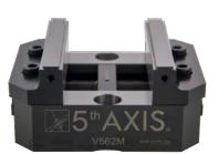
Size: 125.7mm x 152.4mm x 73.6mm Jaw Width: 125.7mm Forward Jaws Clamping Range: 0 - 82.3mm Reverse Jaws Clamping Range: 77.7mm - 153.6mm Clamping Force: 20.0 kN @ 75 Nm Torque Vise Assembly: 75 Nm
