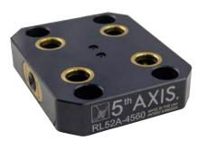
**Size:** 122.0mm x 102.1mm x 25.0mm **Spacing:** 4x M10 or 3/8" @ Ø116mm **Material Construction:** Aluminum (RL52A-4560) Steel (RL52S-4560)
