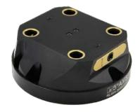
Size: Ø 201.9mm x 75.0mm Spacing: 4x 1/2-13 or M12 bolts @ 90° on Ø 178mm or 3x 1/2-13 or M12 bolts @ 120° on Ø 178mm Material Construction: Aluminum (RL96A-38)
