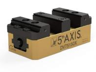
Size: 75mm x 150mm x 56.1mm Jaw Set Material: Hardened Steel 3 Piece Master Jaw Set with Serrated / 45° Dovetail Jaw Width: 75mm Clamping Force: 13.5 kN @ 60 Nm Max Torque: 60 Nm Forward Clamping Range: 0-37.02mm Reverse Clamping Range: 17.23 -55.02mm
