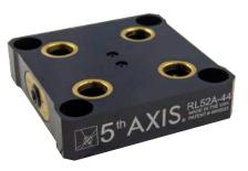
Size: 103.5mm x 103.5mm x 25mm Spacing: 2x SB1210 (Included) and 2x M12 or 1/2" @ Ø82mm 90°. Through hole Ø12.02mm Material Construction: Aluminum (RL52A-44) Steel (RL52S-44)
